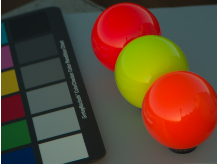
Figure 2: Spheres covered in three different multilayer paint varieties for utility vehicles (“pearl white” primer, fluorescent red/yellow/orange paint, clear coat). Note the outstanding chroma of the paints, and their luminance, which even in the non-specular part is higher than the one of the 90% white ColorChecker patch.
