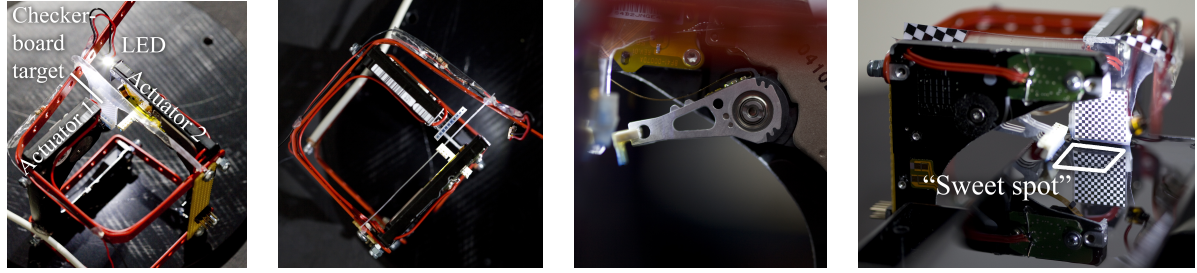
Figure 6: Various views of Setup 2 built from a pair of discarded 2.5-inch hard disk drives. From left to right: Components, top view, close-up on actuator 2, water surface and checkerboard target.
